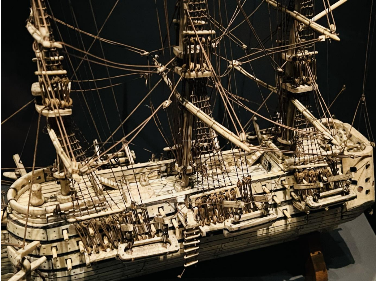
View on deck; six long-boats hoisted in davits; Jacob's ladder
